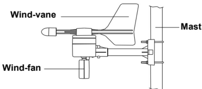
Firstly, check that the wind-fan and the wind-vane can rotate freely before fixing the unit. For correct and accurate readings it is important to mount the sensor so that the front (marked E) is pointing in East-West direction. The wind sensor should now be mounted using the screw provided onto a mast to allow the wind to travel around the sensor unhindered from all directions (ideal mast size should be from  $\varnothing 0.63'' - \varnothing 1.3''$ ).
