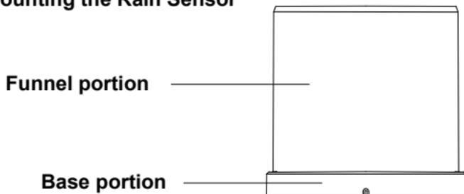
For accurate results, the rain sensor should be securely mounted onto a horizontal surface about 2-3ft above the ground and in an open area away from trees or other coverings where rainfall may be reduced causing inaccurate readings.
