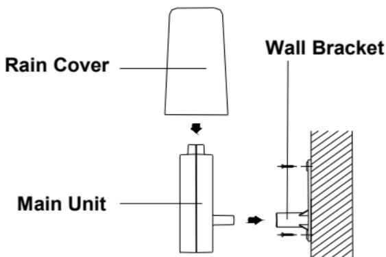
An ideal mounting place for the thermo-hygro sensor would be the outer wall beneath the extension of a roof, as this will protect the sensor from direct sunlight and other extreme weather conditions.
